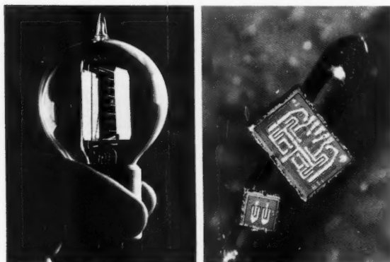
Western Electric's first commercially successful vacuum tube (left) was used in 1915 in the amplifiers that made possible the first transcontinental telephone call. Solid-state electronics, begun at Bell Labs, makes it possible for tiny integrated circuits (right) to do the work of many vacuum tubes.
